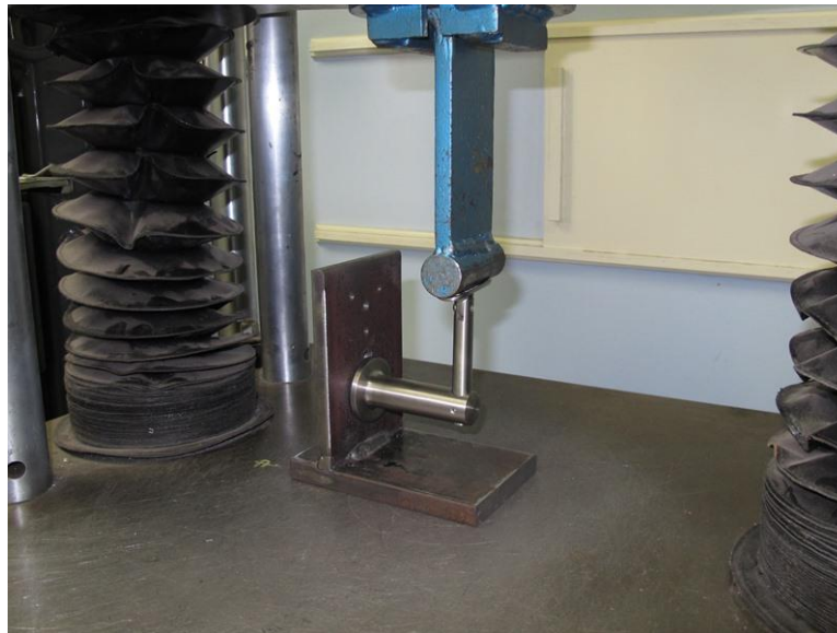
Handrail bracket under the test
