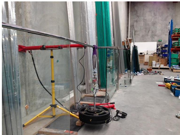
25.4mm round slotted tube under the test
