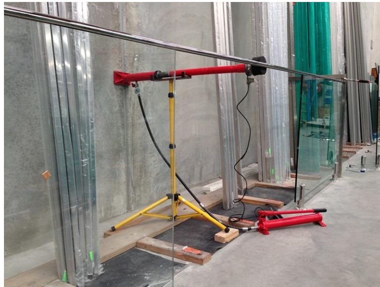
The test arrangement with 25.4mm round slotted handrail under the test.
