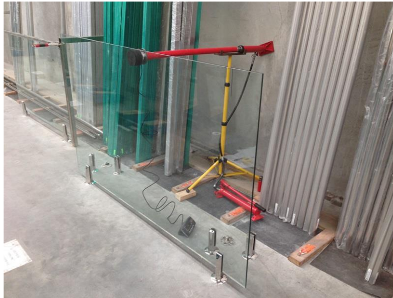
Diamond Core Drilled spigots under the test
