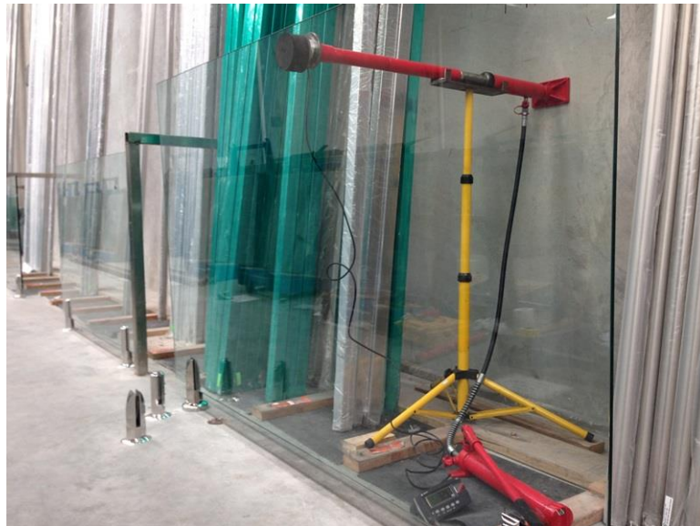
Diamond Deck mounted spigots under the test
