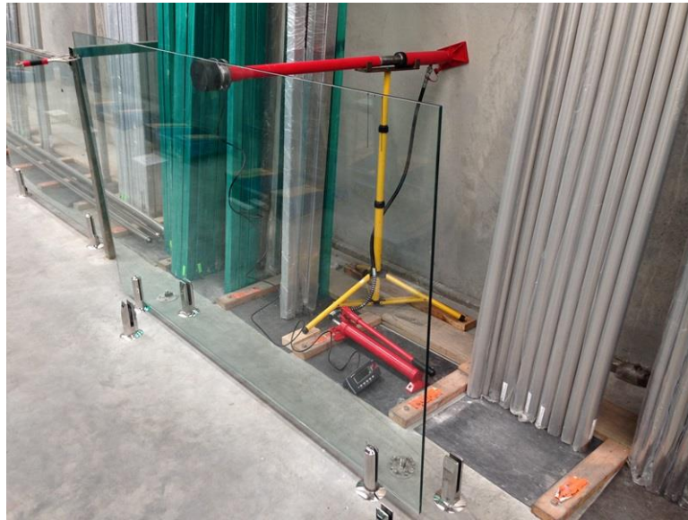
Round Core Drilled spigots under the test
