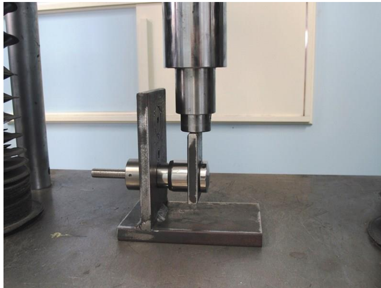
The standoff fitting under the test
