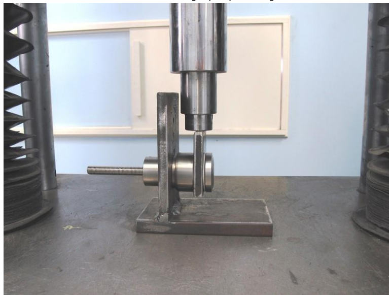
The standoff fitting under the test
