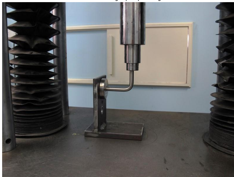
Handrail bracket under the test
